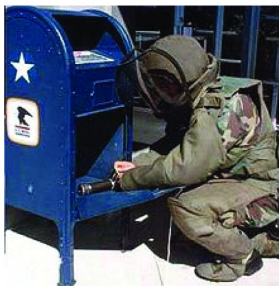
Figure 7. Bomb suits use ice for coolant because they prevent thermoregulation by evaporation of perspiration (reproduced from reference (57)).
