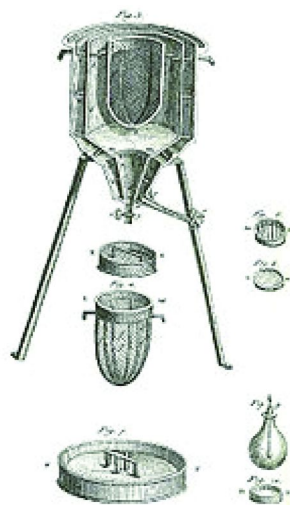
Figure 1. The original ice-calorimeter, used by Antoine Lavoisier and Pierre-Simon Laplace in 1782-83, to investigate Joseph Black's prior discovery of latent heat (reproduced from reference (51)).
